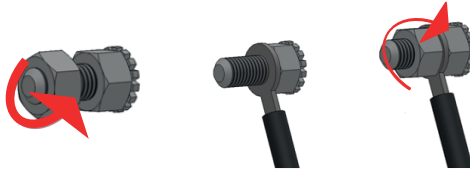
Figure 5. Connection of the device with installation of equalising electrical potentials.
